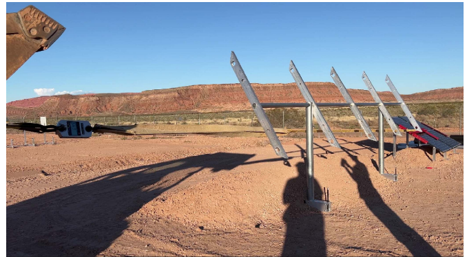
Photo 4: Horizontal force test at max load
