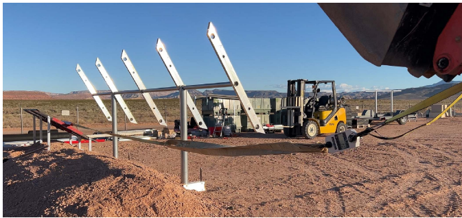
PHOTO 1: Horizontal force test setup
