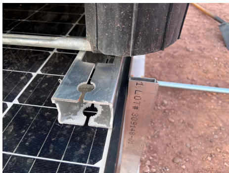
PHOTO 7: Slight deflections noted under load
