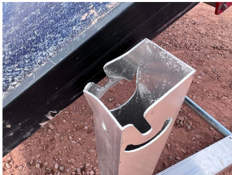
PHOTO 14: Upright mount deformation after testing
