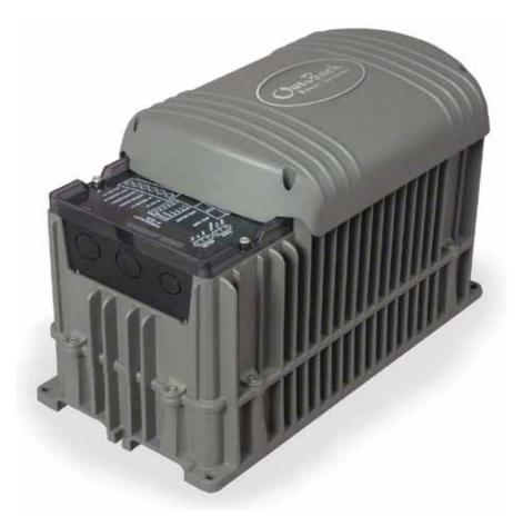
The OutBack true sinewave GFX International Series Inverter/ Charger is a competitive power solution designed for applications with lower power demands. Incorporating a DCto-AC sinewave inverter, battery charger and AC transfer relay housed within a die-cast aluminum chassis, the International Series GFX Inverter/Chargers give you the ability to sell solar, wind or hydro power back to the utility grid while providing instantaneous back-up power in the event of a utility outage.
