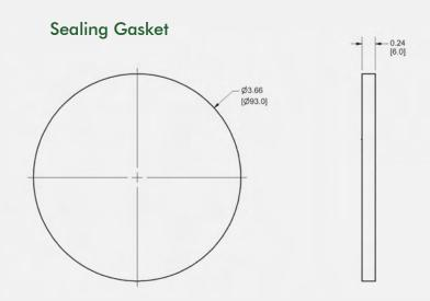
Material: Aluminum and Neoprene Gasket with Mastic Tape
