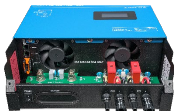
Inside the SmartSolar MPPT RS 450|100
