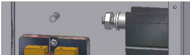
5/16" stud for battery negative tie point
