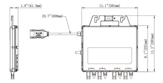
The APsystems QS1 is a grid-tied microinverter with intelligent networking and advanced monitoring systems to ensure maximum efficiency. High efficiency, high reliability of the QS1 with 4 independent MPPT inputs, Maximum AC output power reaching 1200W. Quarter the inverters and quarter the installation means real cost savings for residential and commercial customers.
