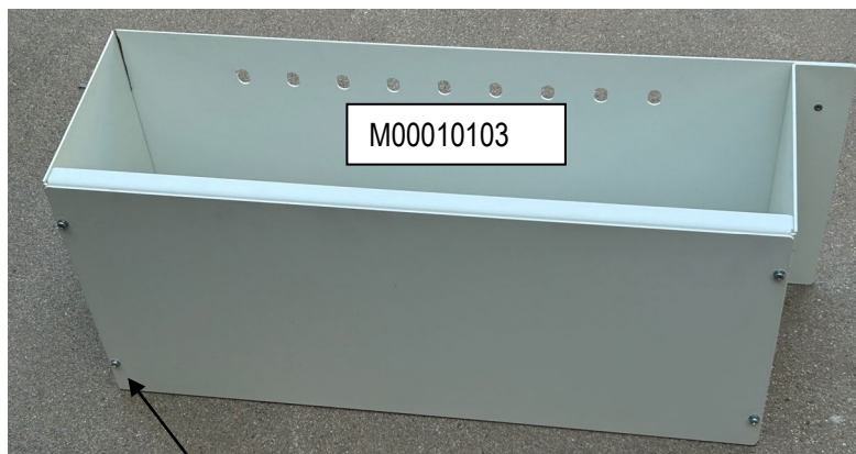
8-32 Steel Pan Head Screws with Spring Lock Washer
