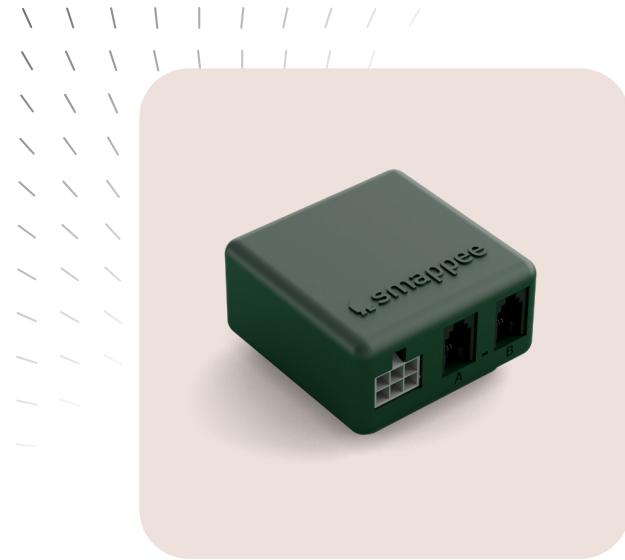
The Power Box is the compact and robust heart of the Smappee Infinity monitoring system. It's compatible with almost any electricity network worldwide and is DIN-rail mountable. It measures the line voltage of the connected phases, collects the currents from the CT sensors and calculates power, active energy, reactive energy and other energy and power quality data. It also provides power to all components.
