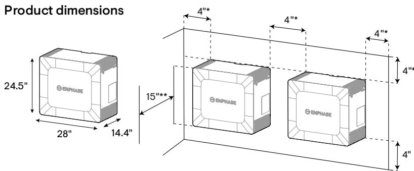
\* The 4" clearances on the sides and the top are per the UL 9540A evaluation. Enphase recommends 8" for ease of service.
