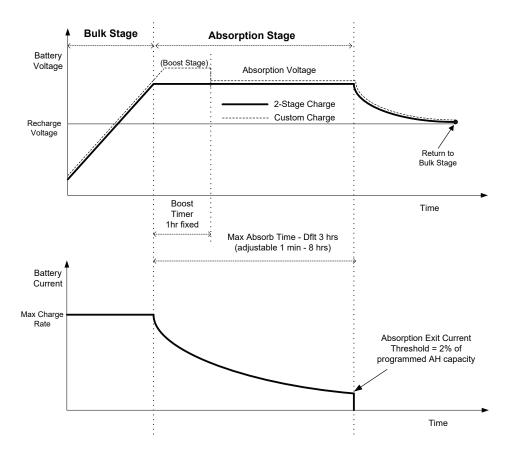
Figure 16 Two-Stage Charging Cycle
