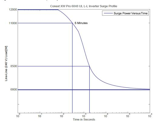
Figure 28 AC Overload Capability
