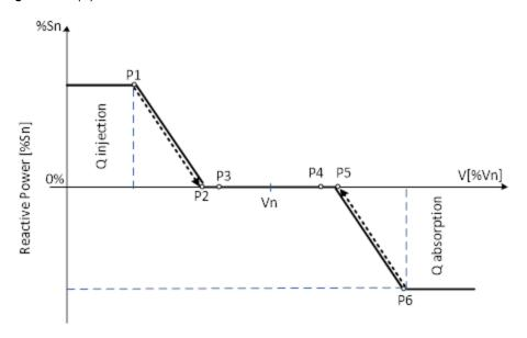
Q – The Conext XW Pro output reactive power in percentage of nominal rated apparent power Sn.
