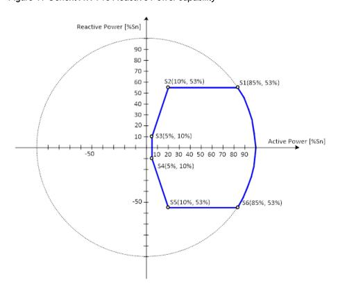
Figure 41 Conext XW Pro Reactive Power capability
