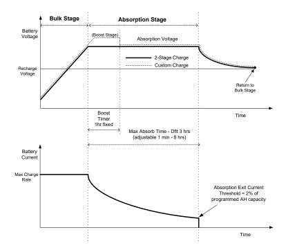
Figure 15 Three-Stage Battery Charging Cycle
