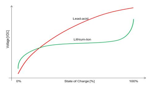
The battery SOC is typically calculated by a third-party Battery Management System, Conext Battery Monitor, or any other external device with such a function. The BMS also ensures safe operation of the batteries by establishing operational limits for the attached inverter-charger unit.
