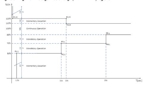
Figure 54 High/Low Voltage Ride-through (HVRT/LVRT) regions
