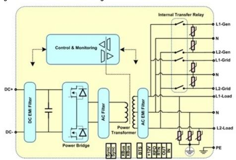
Figure 26 Conext XW Pro Block Diagram
