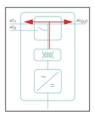
Figure 8 AC Passthrough
