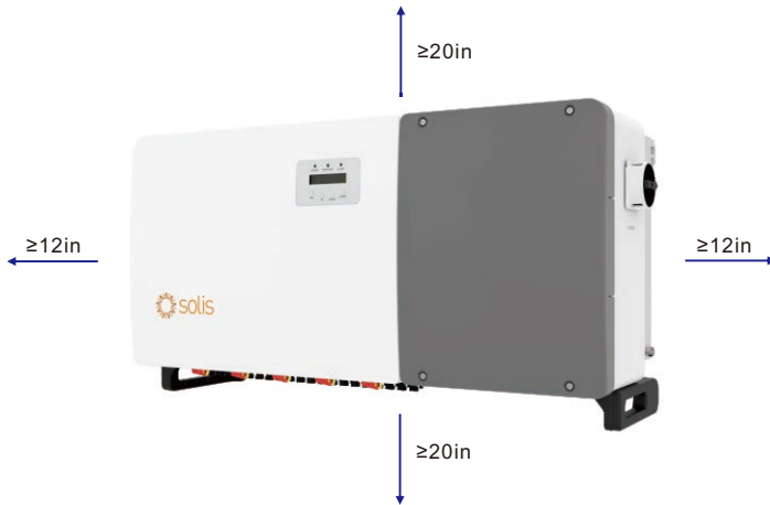
Figure 3.2 Clearance distances requirement for the inverter
