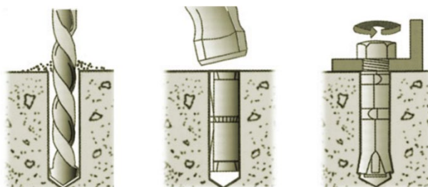
Figure 4-8 Drill holes, set Anchors, and tighten Assembly Bolts
