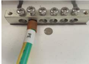
Figure 4.10 Grounding Terminal on Heat-Sink
