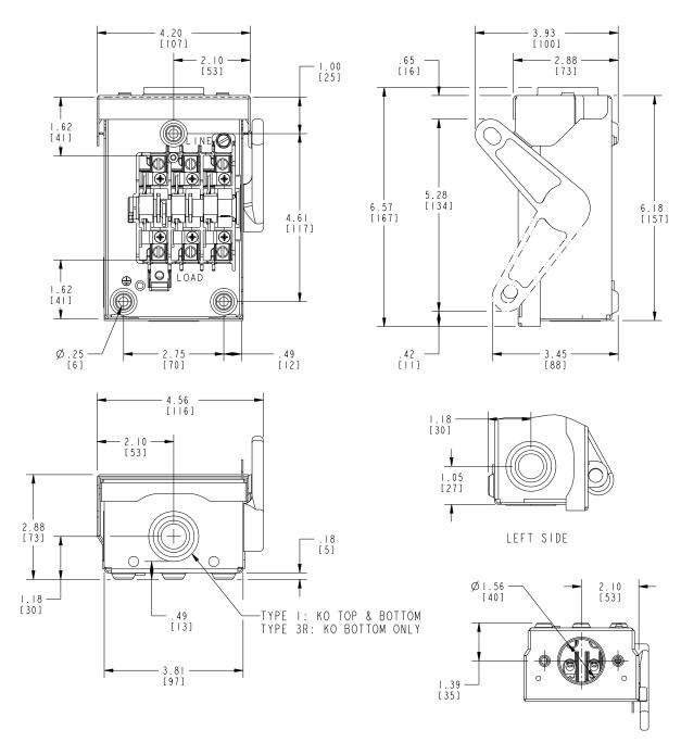
TYPE I ENCLOSURES: COLD ROLLED STEEL .045" THICK FINISH: ANSI GREY #61 PAINT
