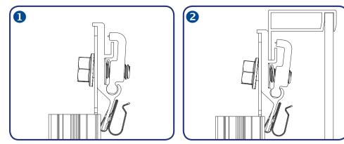
3. Tighten the mounting bolt on the MLPE Frame Attachment Kit to 10 lb-ft (120 lb-in).
