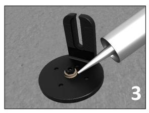
Apply a copious amount of sealant around the Lag Screw and Sealing Washer of the NanoMount.
