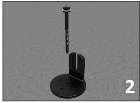
Locate the center of the rafter in the desired roof location and drill a 7/32" [6mm] pilot hole. Clear away any debris before filling the pilot hole with sealant.
