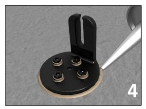
Apply a copious amount of sealant around the base of the NanoMount.
