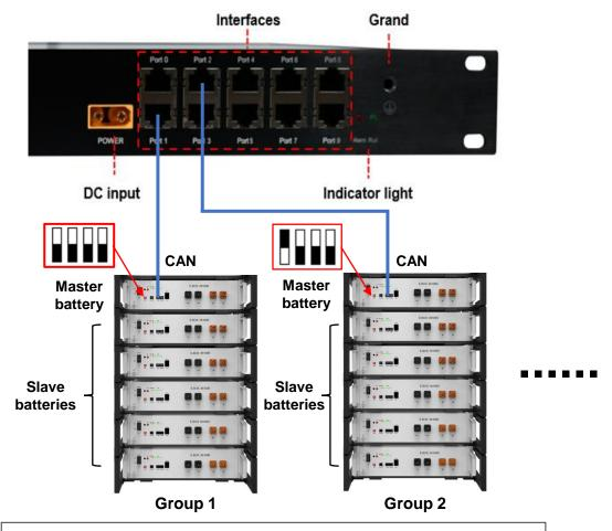
No special requirement for the DIP Switch setting of the Slave batteries
