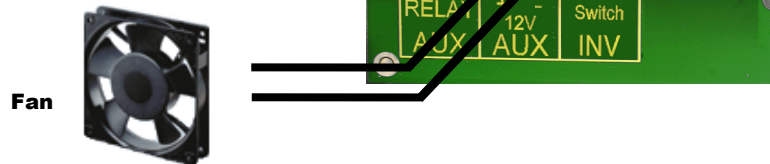
Figure 21 AUX Connections for Vent Fan (Example)
