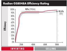
Typical Efficiency Rating: Real world efficiency with variable loads • GS8048A: 93% CEC Efficiency Rating: Most stringent US rating • GS8048A: 92.5%
