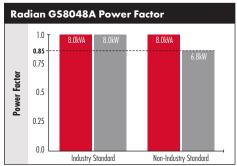
Power Rating Notes: Inverters that specify power in VA but do not use the unity standard Power Factor (PF) could have misleading power specifications. Volt-amps (VA) is a total inverter output, while warts (W) represent the power consumed by the electrical loads. PF, which varies by types of loads, is the ratio of W to VA, and the difference between the two is power in the circuit that does no useful work. At 1.0PF (unity), all power is used. This is the industry standard used by OutBack Power".
