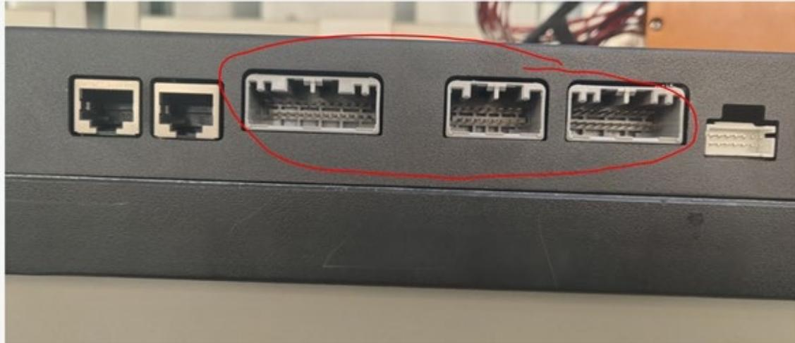
6. After ~ 60 Mins: use multi-meter to read battery cell voltage from the plug. You will need fine/thin probe leads to analyze voltage in this manner.
