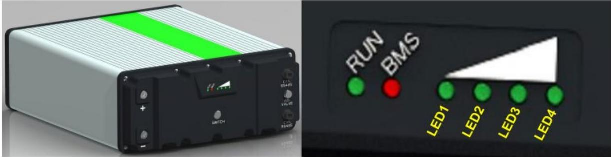
The red “BMS” light will turn on during start-up diagnostic as well as when there is a communication error between batteries. If the problem persists, please fill out a support ticket at <https://support.fortresspower.com> .
