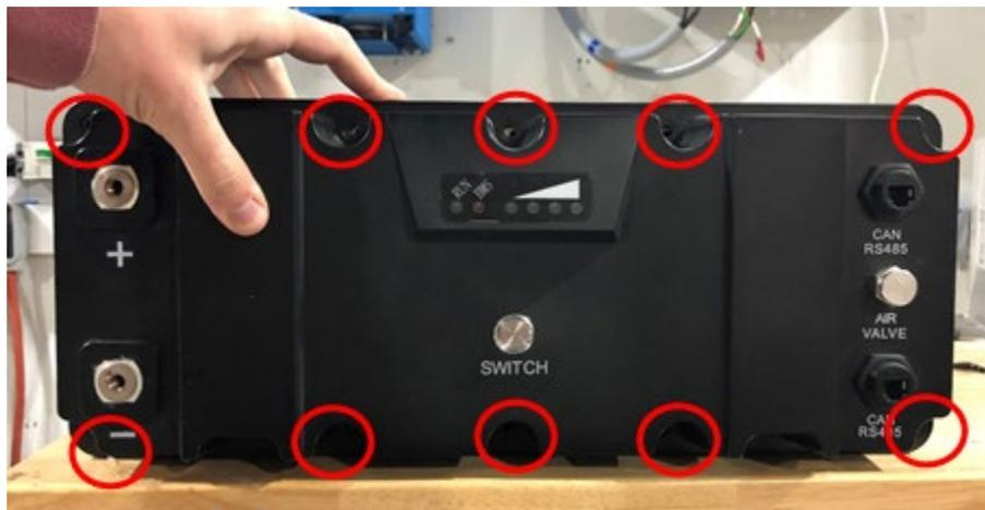
3. eFlex with serial number 2205## (made in May 2022 onward) contain a gasket lid, which can be easily removed after the screw removal.
