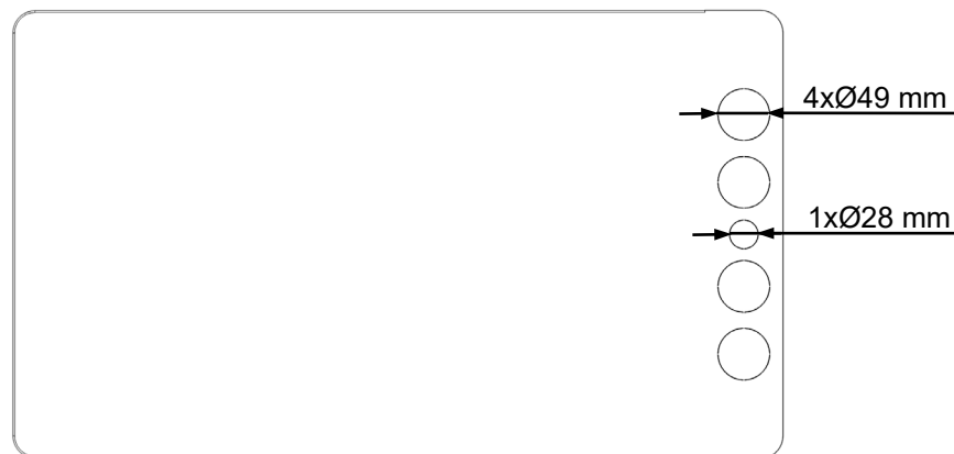
Figure 9: Control Module Knockout Details
