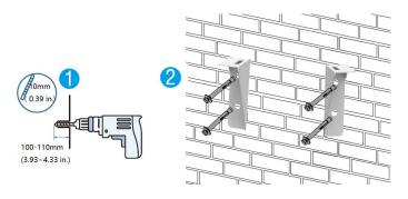
4. Carry the battery and secure the battery to the wall-mounted brackets using 4 sets of M6 screws and buckle nuts.
