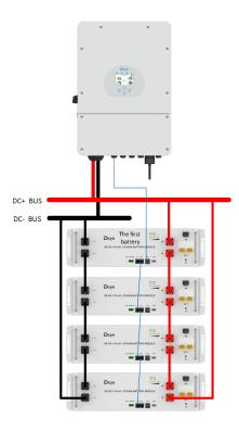
**5.2.2 Mode 2** Schematic diagram of parallel connection of high-power system batteries:
